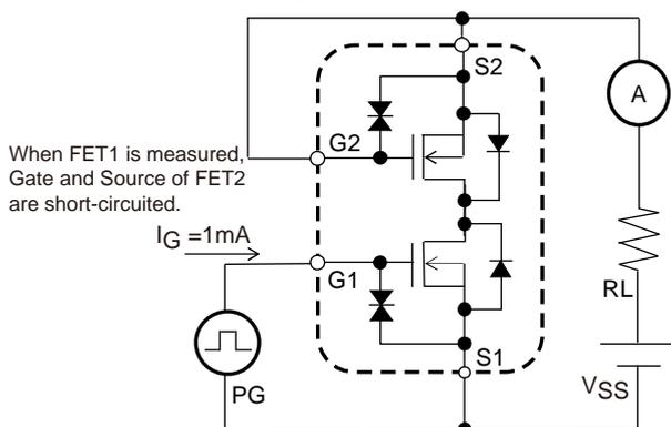
When FET1 is measured, Gate and Source of FET2 are short-circuited.
