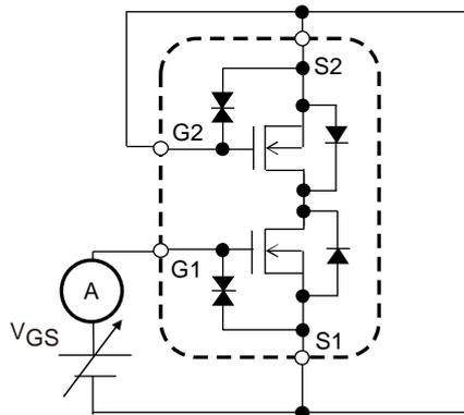
When FET1 is measured, Gate and Source of FET2 are short-circuited.
