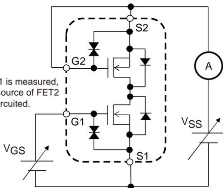
When FET1 is measured, Gate and Source of FET2 are short-circuited.
