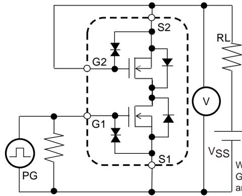
When FET1 is measured, Gate and Source of FET2 are short-circuited.
