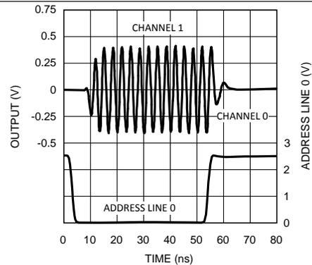
Figure 12. Channel Switching
