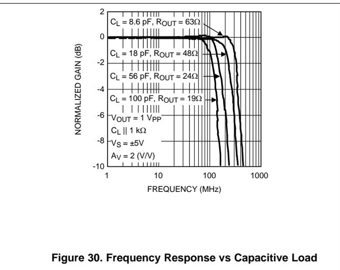
Figure 30. Frequency Response vs Capacitive Load
