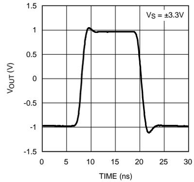
Figure 8. Pulse Response 2V<sub>PP</sub>
