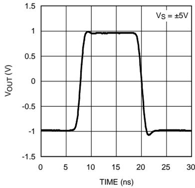
Figure 7. Pulse Response 2V<sub>PP</sub>
