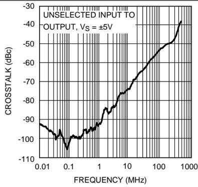
Figure 25. Crosstalk vs Frequency
