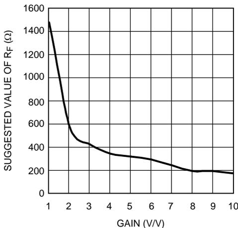
Figure 27. Suggested R<sub>F</sub> vs Gain
