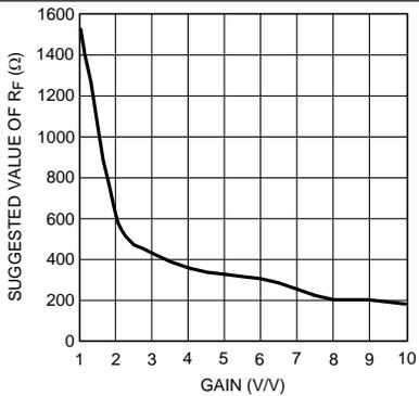
Figure 5. Suggested Value of  $R_F$  vs Gain
