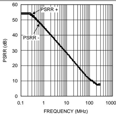
Figure 11. PSRR vs Frequency
