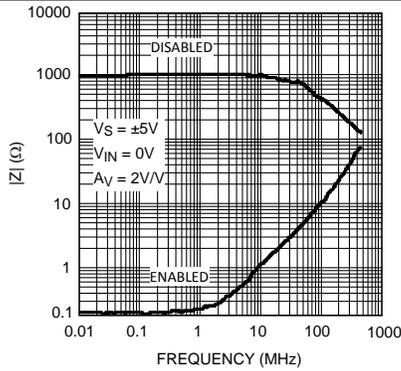
Figure 9. Closed Loop Output Impedance
