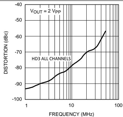
Figure 18. HD3 vs Frequency
