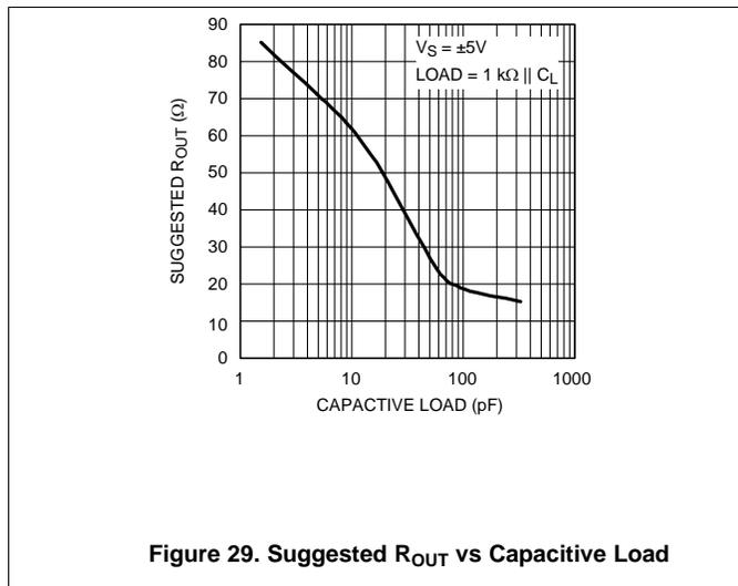
Figure 29. Suggested  $R_{OUT}$  vs Capacitive Load
