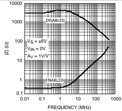
Figure 10. Closed Loop Output Impedance
