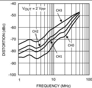
Figure 17. HD2 vs Frequency
