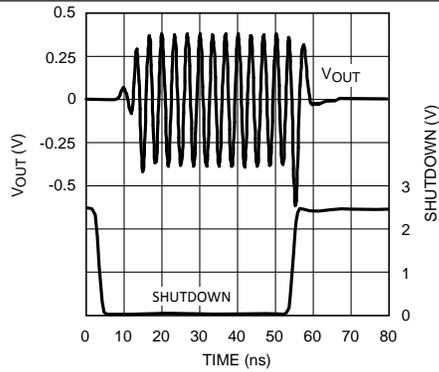
Figure 13. SHUTDOWN Switching
