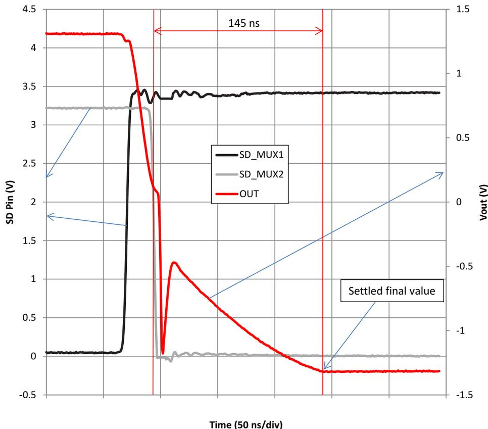
Figure 33. SD Pin Switching Waveform and Output Settling
