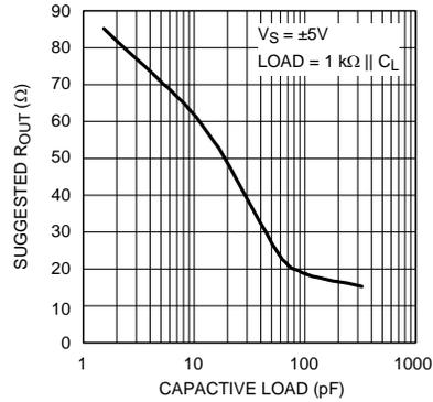
Figure 4. Suggested  $R_{OUT}$  vs Capacitive Load
