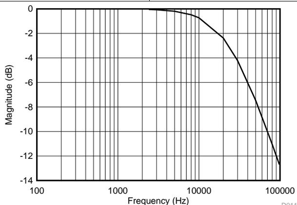
R1 = 10-k $\Omega$  pullup resistor, C2 = 680 pF
