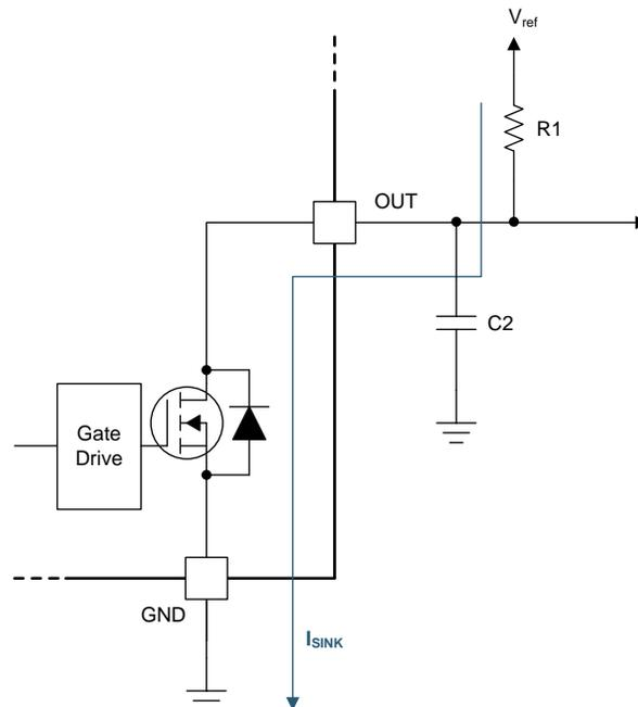
Figure 19. Open-Drain Output
