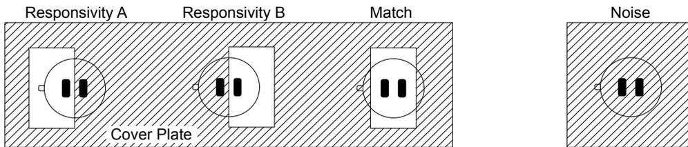
The typical set-up for the measurement of responsivity and match is illustrated in figure 2. The black body (BB) radiator (1) is set to 373 K (100 °C). The signal is modulated by a rotating chopper (2). An aperture (3) is used to adjust the radiation flux. The cover plate (4) is masking the elements as shown in figure 3. The sensor (5) is interfaced to a signal processing chain (6). To measure noise, a bandpass filter in the range of 0.4 Hz to 10 Hz is applied.
