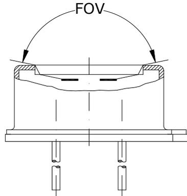
The horizontal field of view (FOV) as drawn to figure 4 is given as the geometrically unobstructed light path to both elements. The FOV of 100° is given for the optical light acceptance with the full so-called common mode suppression.
