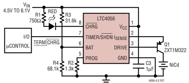
Figure 7. Nickel Chemistry Battery Charging
