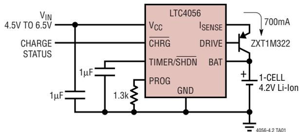
**V<sub>IN</sub> Undervoltage Charge Current Limiting**
