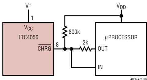
Figure 2. Using a Microprocessor to Determine  $\overline{CHRG}$  State
