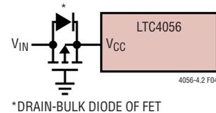
Figure 4. Low Loss Input Reverse Polarity Protection
