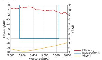
• Tested antenna has been soldered. Evaluation board size is 120x65x1 mm.
