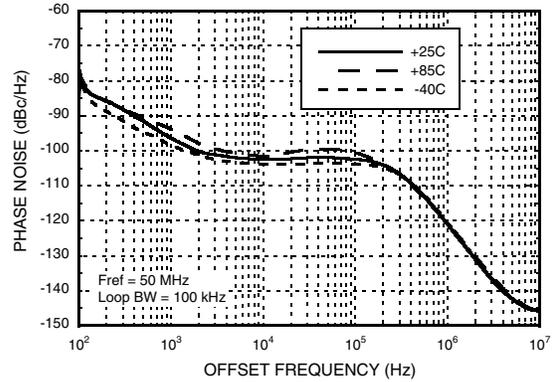
**SSB Phase Noise Fractional Spurs @ 7.802 GHz**
