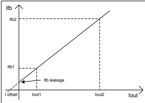
The current sensing is specified by measuring 3 points :
