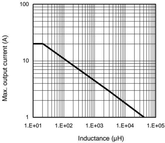
**Figure 9 – Max. Iout (A) Vs inductance (µH)**
