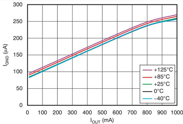
Figure 11. Ground Pin Current vs Load Current
