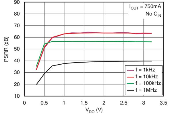
Figure 20. Power-Supply Ripple Rejection vs Dropout Voltage
