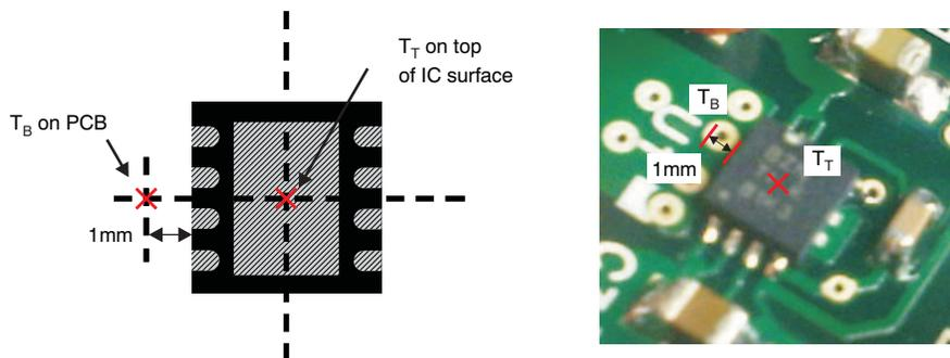
**Figure 36. Measuring Points for  $T_T$  and  $T_B$**
