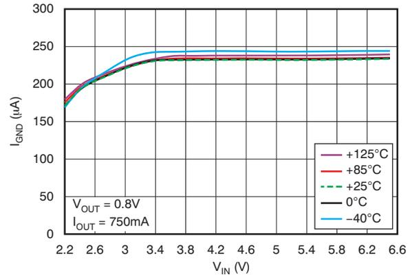
Figure 10. Ground Pin Current vs Input Voltage
