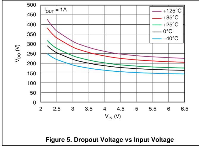
Figure 5. Dropout Voltage vs Input Voltage
