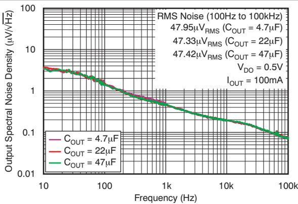
Figure 21. Output Spectral Noise Density vs Frequency
