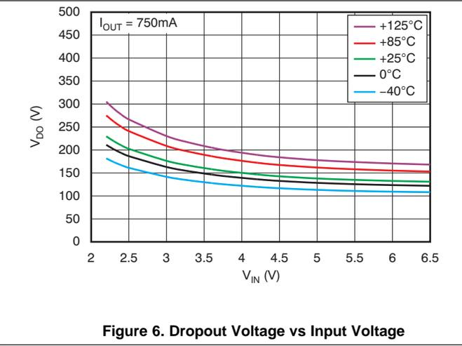
Figure 6. Dropout Voltage vs Input Voltage
