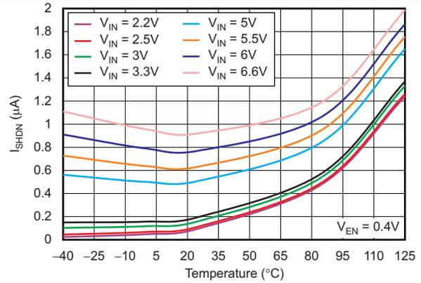
Figure 12. Shutdown Current vs Temperature
