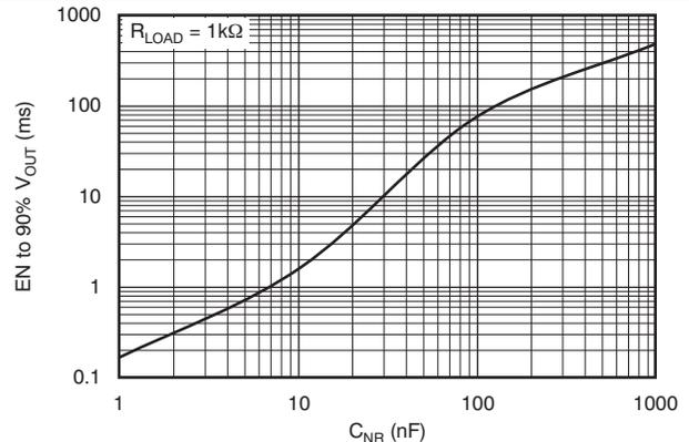
Figure 24. Start-Up Time vs Noise Reduction Capacitance
