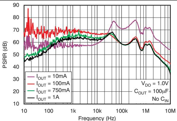
Figure 17. Power-Supply Ripple Rejection vs Frequency
