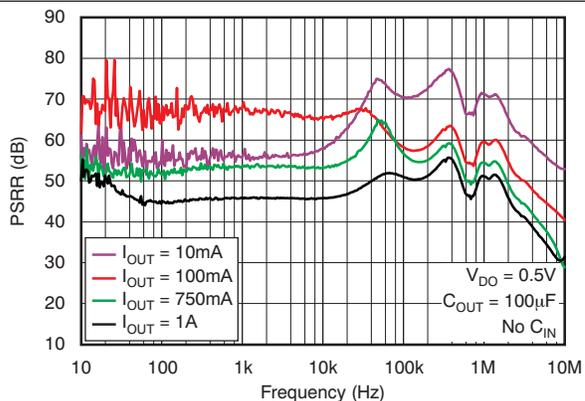
Figure 18. Power-Supply Ripple Rejection vs Frequency
