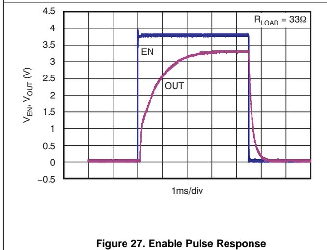
Figure 27. Enable Pulse Response
