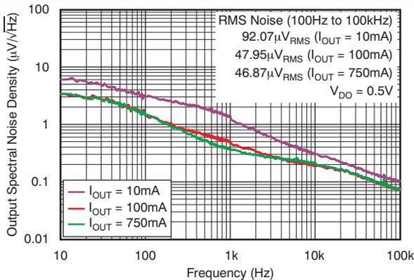
Figure 23. Output Spectral Noise Density vs Frequency
