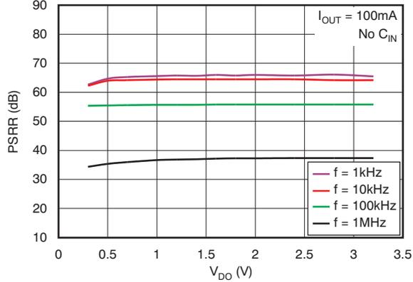
Figure 19. Power-Supply Ripple Rejection vs Dropout Voltage
