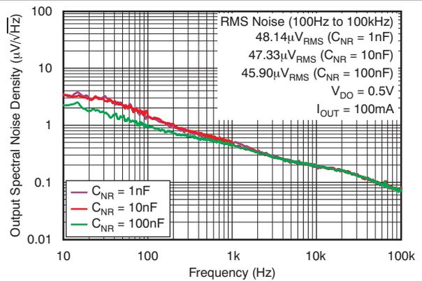
Figure 22. Output Spectral Noise Density vs Frequency
