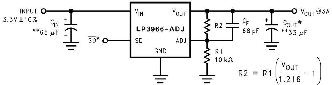
\*SD and ERROR pins must be pulled high through a 10kΩ pull-up resistor. Connect the ERROR pin to ground if this function is not used. See [Application Hints](#) for more information.
