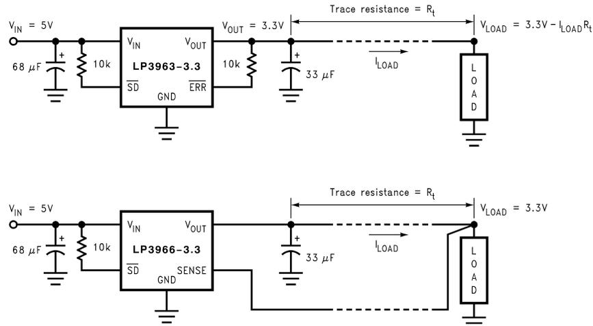
Figure 22. Improving remote load regulation using LP3966
