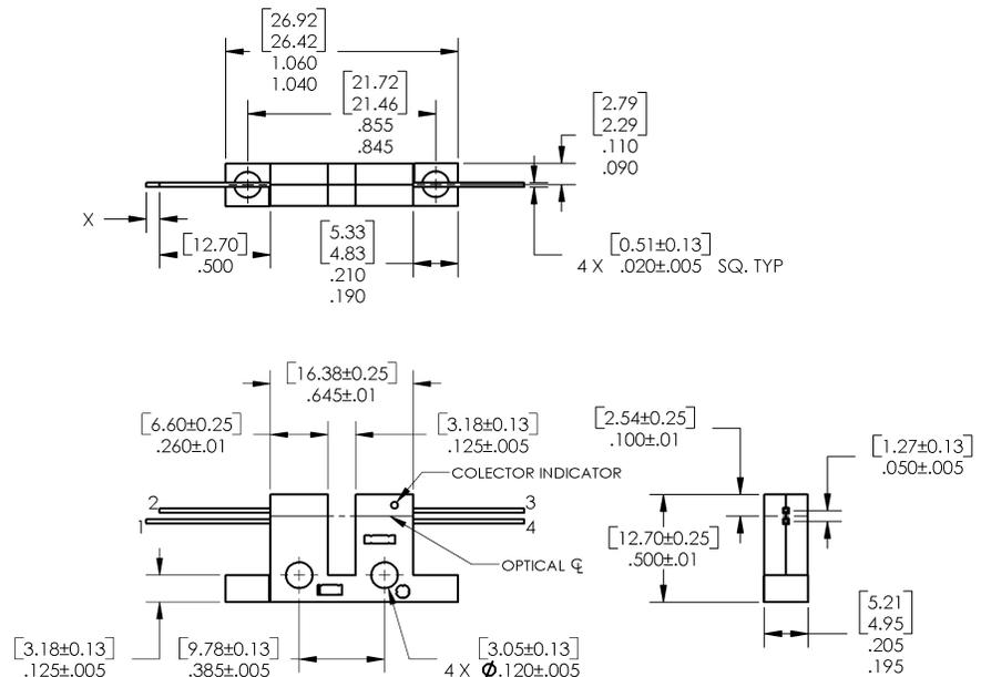
DIMENSIONS ARE IN: [ MILLIMETERS ]
