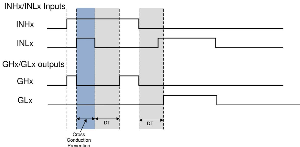
**Figure 7-2. Cross Conduction Prevention and Deadtime Insertion**
