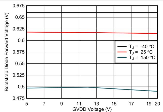
Figure 6-4. Bootstrap Diode Forward Voltage over GVDD Voltage
