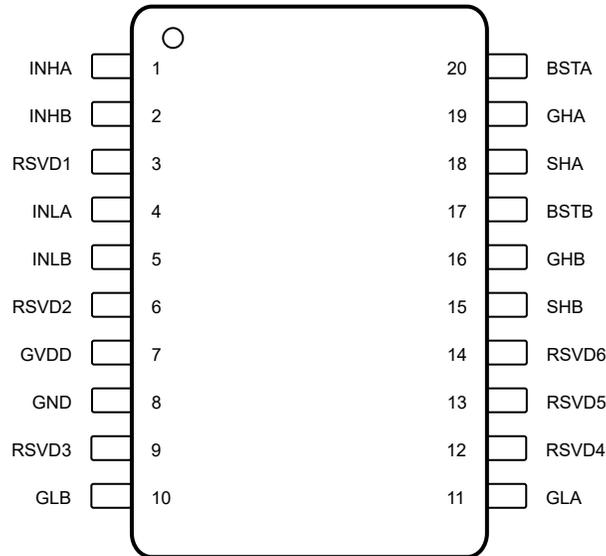
Figure 5-2. DRV8770 PW Package 20-Pin TSSOP Top View
