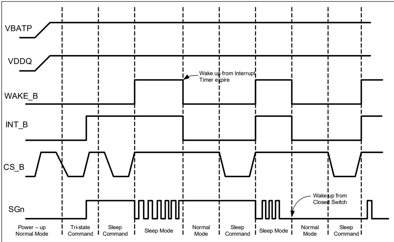
**Figure 17. Low-power mode to Normal mode operation**
