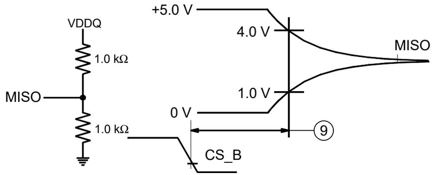
Figure 8. MISO loading for disable time measurement
