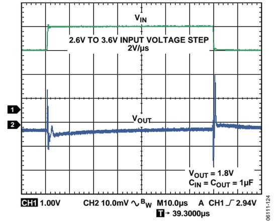
Figure 22. Line Transient Response, Load Current = 300 mA
