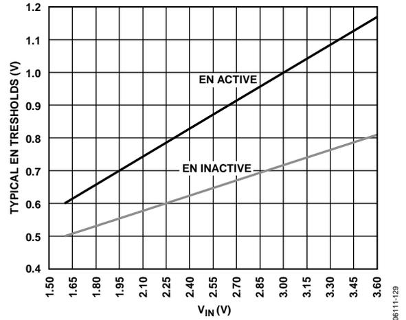
Figure 28. Typical EN Pin Thresholds vs. Input Voltage
