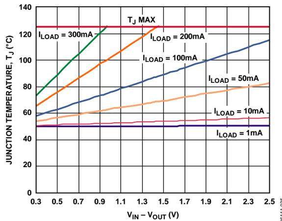
Figure 35. 0 mm<sup>2</sup> of PCB Copper, T<sub>A</sub> = 50°C
