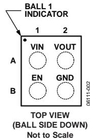
Figure 2. Pin Configuration
