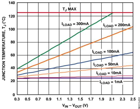
Figure 31. 100 mm<sup>2</sup> of PCB Copper, T<sub>A</sub> = 25°C
