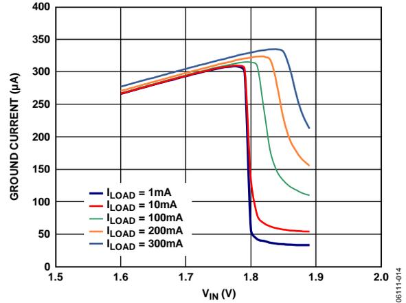
Figure 12. Ground Current vs. Input Voltage (in Dropout)
