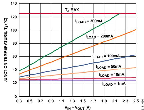
Figure 30. 500 mm<sup>2</sup> of PCB Copper,  $T_A = 25^\circ\text{C}$
