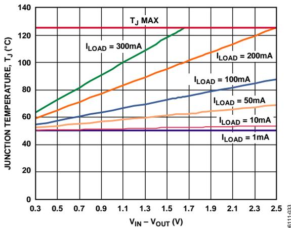
Figure 33. 500 mm<sup>2</sup> of PCB Copper, T<sub>A</sub> = 50°C
