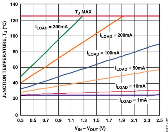
Figure 32. 0 mm<sup>2</sup> of PCB Copper, T<sub>A</sub> = 25°C
