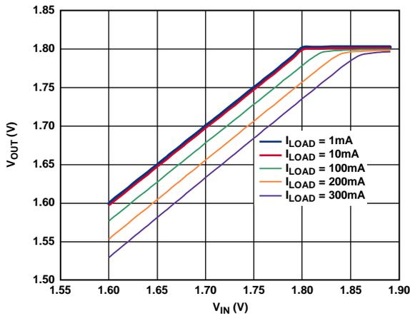
Figure 11. Output Voltage vs. Input Voltage (in Dropout)
