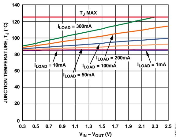
Figure 36. T<sub>A</sub> = 85°C
