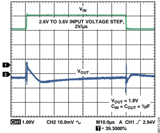
Figure 21. Line Transient Response, Load Current = 1 mA
