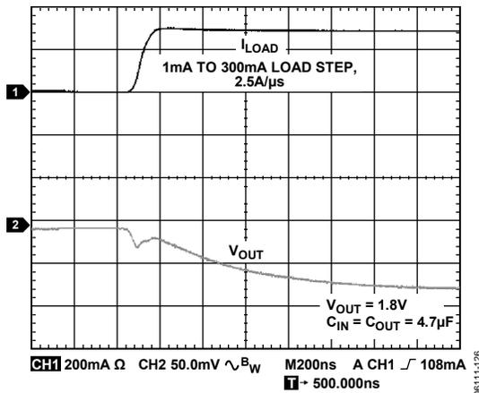
Figure 25. Output Transient Response,  $C_{OUT} = 4.7 \mu\text{F}$
