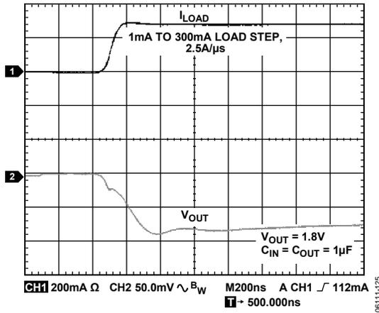
Figure 24. Output Transient Response,  $C_{OUT} = 1 \mu\text{F}$
