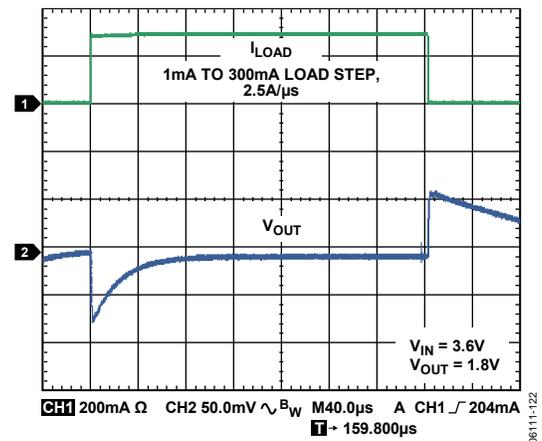
Figure 20. Load Transient Response,  $C_{IN}$  and  $C_{OUT} = 4.7\ \mu\text{F}$
