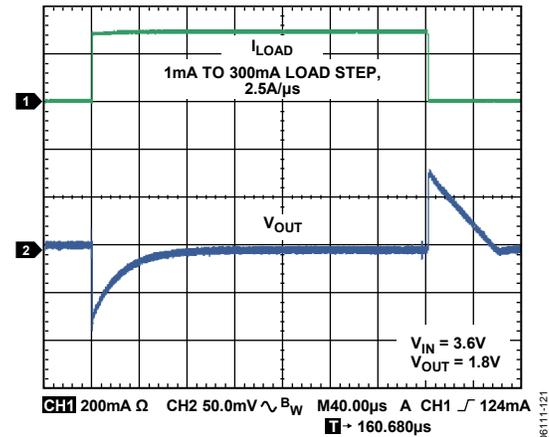
Figure 19. Load Transient Response,  $C_{IN}$  and  $C_{OUT} = 1\ \mu\text{F}$
