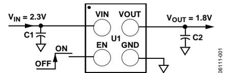
Figure 1. [ADP172](#) with Fixed Output Voltage, 1.8 V
