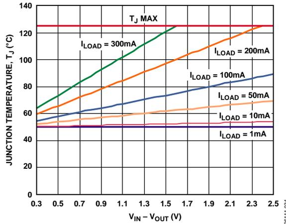
Figure 34. 100 mm<sup>2</sup> of PCB Copper, T<sub>A</sub> = 50°C
