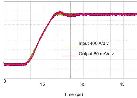
Figure 2: Typical delay time (0 to 2 kA, 400 A/μs)
