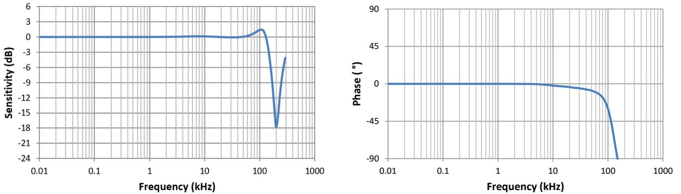
Figure 5: Typical frequency response, small signal bandwidth
