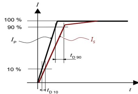
Figure 6:  $t_{D10}$  (delay time @ 10 %) and  $t_{D90}$  (delay time @ 90 %)
