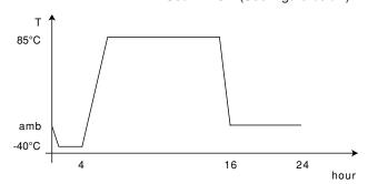
Thermal Shock . . . . . . . According to SAE J1455, Sec. 4.1.3.2 (see Fig)
