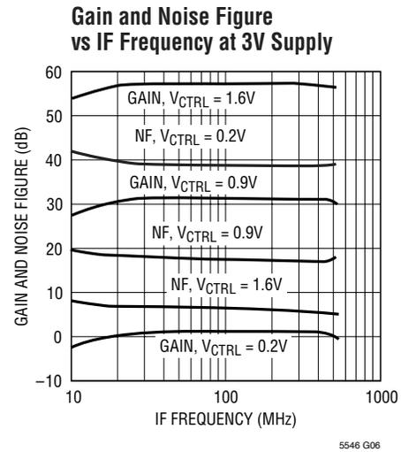
**TYPICAL PERFORMANCE CHARACTERISTICS**  $V_{CC} = 3V$ ,  $f_{2 \times LO} = 570MHz$ ,  $P_{2 \times LO} = -5dBm$
