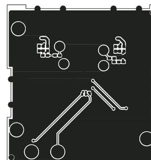
Figure 10. Bottom Side Layout of Evaluation Board
