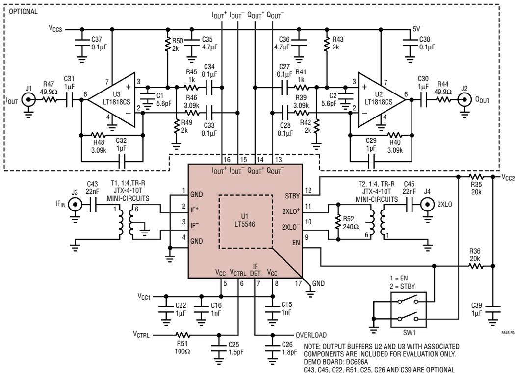
**Figure 6. Evaluation Circuit Schematic with I/Q Output Buffers**
