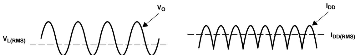
**Figure 36. Voltage and Current Waveforms for BTL Amplifiers**
