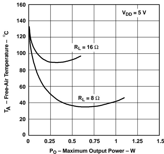
**Figure 39. Free-Air Temperature vs Maximum Continuous Output Power**
