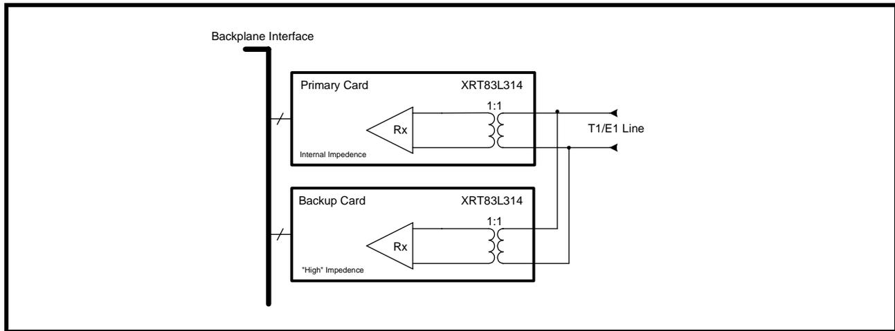
**4.3.4 N+1 Redundancy Using External Relays**
