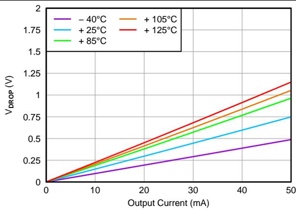
Figure 7. Dropout Voltage
