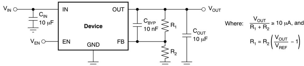
Figure 13. Example Circuit to Maximize Transient Performance
