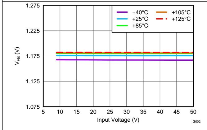
Figure 3. Feedback Voltage
