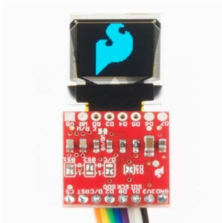
The Micro OLED Breakout Board breaks out a small monochrome, blue-on-black OLED. It's 64 pixels wide and 48 pixels tall, measuring 0.66" across. It's micro, but it still packs a punch – the OLED display is crisp, and you can fit a deceptively large amount of graphics on there. Most important of all, though, is the Micro OLED is easy to control over either an SPI or I<sup>2</sup>C interface.
