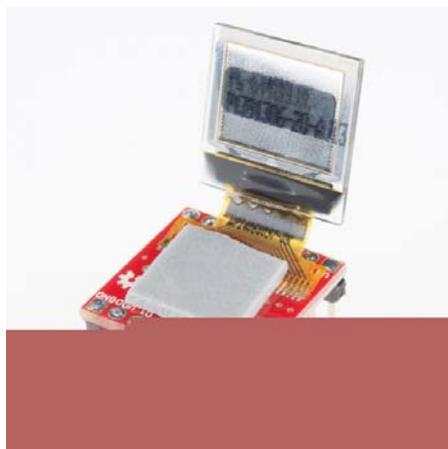
Fold the display over and it should fit perfectly within the PCB's outline.
