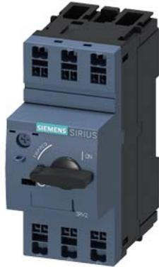
Circuit breaker size S00 for transformer protection A-release 1.8...2.5 A N release 52 A Spring-type terminal Standard switching capacity
