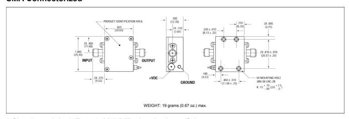
5. Dimensions are inches (millimeters) ±0.015 (0.38) unless otherwise specified.
