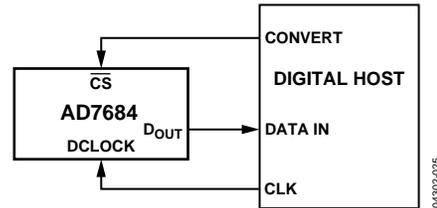
Figure 25. Connection Diagram
