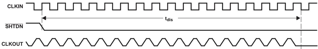
Figure 8. Disable Time Waveforms (CLKSEL low shown)
