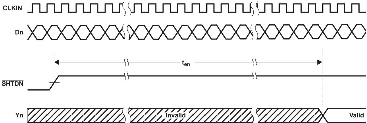
Figure 7. Enable Time Waveforms (CLKSEL low shown)
