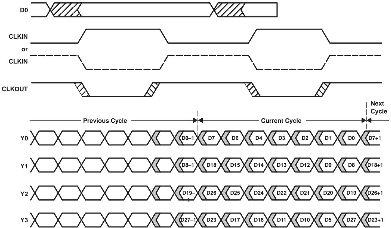
Figure 1. Typical LVDS93 Load and Shift Sequences
