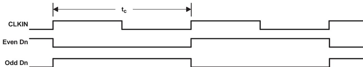
NOTE A: The worst-case test pattern produces nearly the maximum switching frequency for all of the LVDS outputs. Pattern with CLKSEL low shown.
