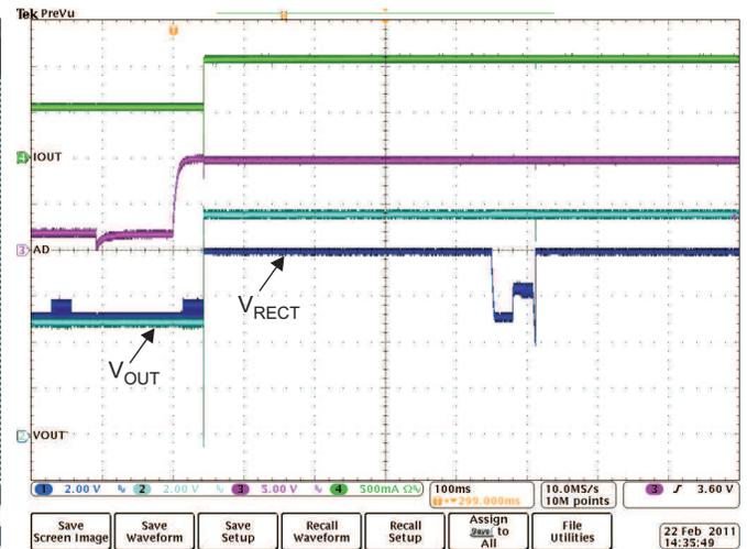
**Figure 17. Adapter Insertion ( $V_{AD} = 10\text{V}$ )**
