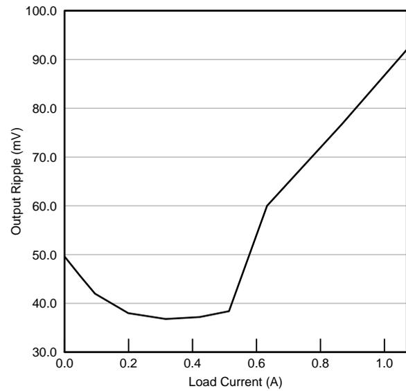
**Figure 9. Output Ripple vs.  $I_{LOAD}$  ( $C_{OUT} = 1\mu F$ )**
