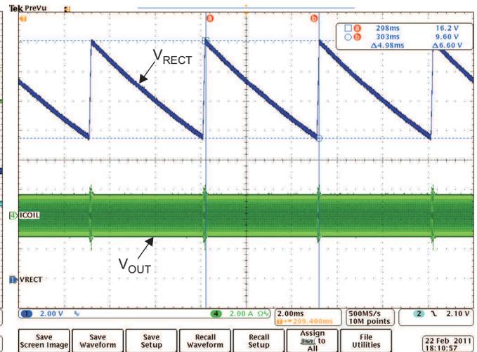
**Figure 15. Rectifier Overvoltage Clamp ( $f_{op} = 110\text{kHz}$ )**
