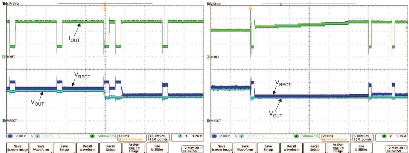
Figure 22. bq51011 Output Voltage Transition (V<sub>OUT</sub> = 4.8V -> 3.5V) Illustrating V<sub>RECT-TRACK</sub>
