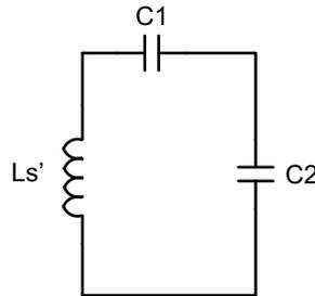
**Figure 30. Dual Resonant Circuit with the Receiver Coil**
