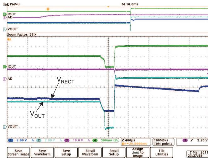
Figure 18. Adapter Insertion ( $V_{AD} = 10V$ ) Illustrating Break-Before-Make Operation
