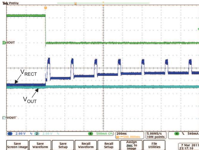
**Figure 14. 1A Load Dump Full System Response**
