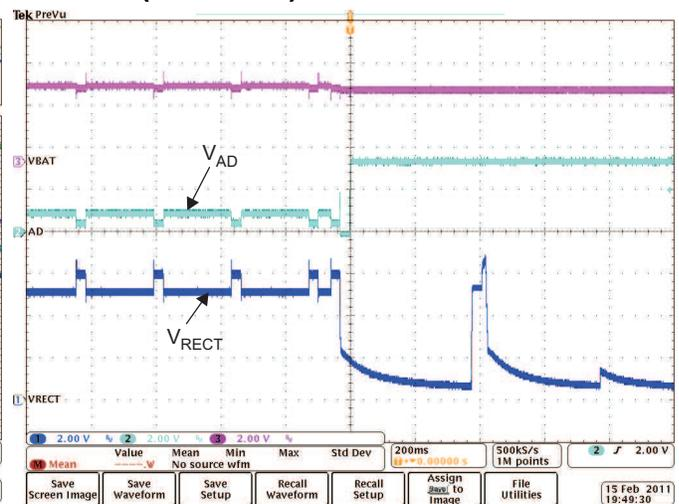
Figure 19. On the Go Enabled ( $V_{OTG} = 3.5V$ )(3)
