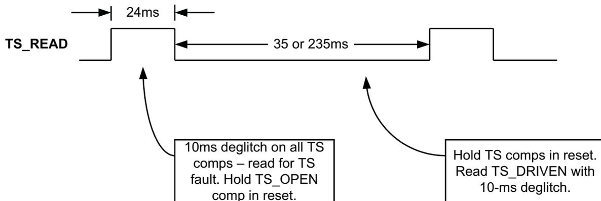
Figure 29. Timing Diagram for TS Detection Circuit
