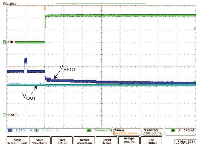
Figure 13. 1A Load Step Full System Response
