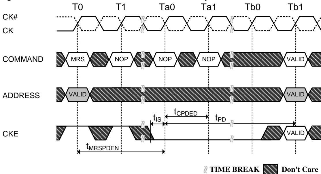
**Figure 65. Synchronous ODT Timing Example**
