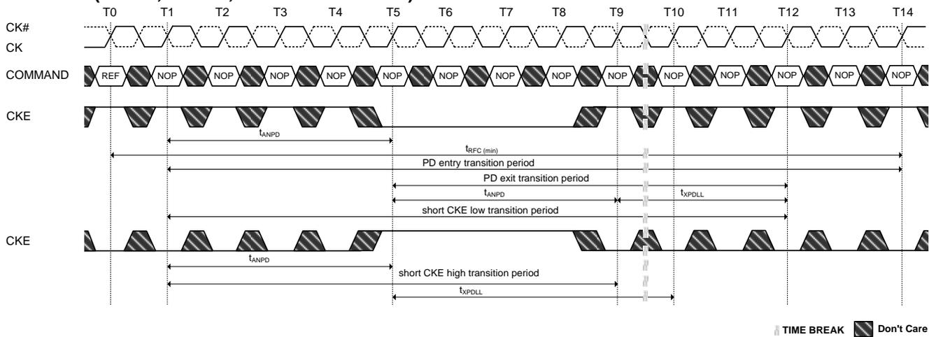
**Figure 77. Power-Down Entry,Exit Clarifications-Case 1**
