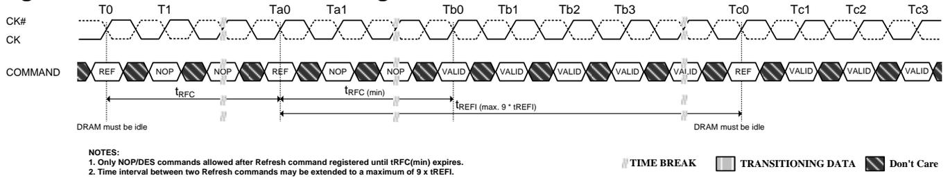
**Figure 54. Self-Refresh Entry/Exit Timing**
