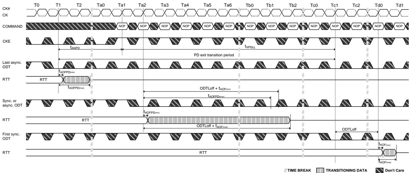
**Figure 76. Transition period for short CKE cycles, entry and exit period overlapping**
