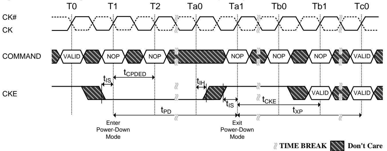
**Figure 60. Precharge Power-Down (Slow Exit Mode) Entry and Exit**
