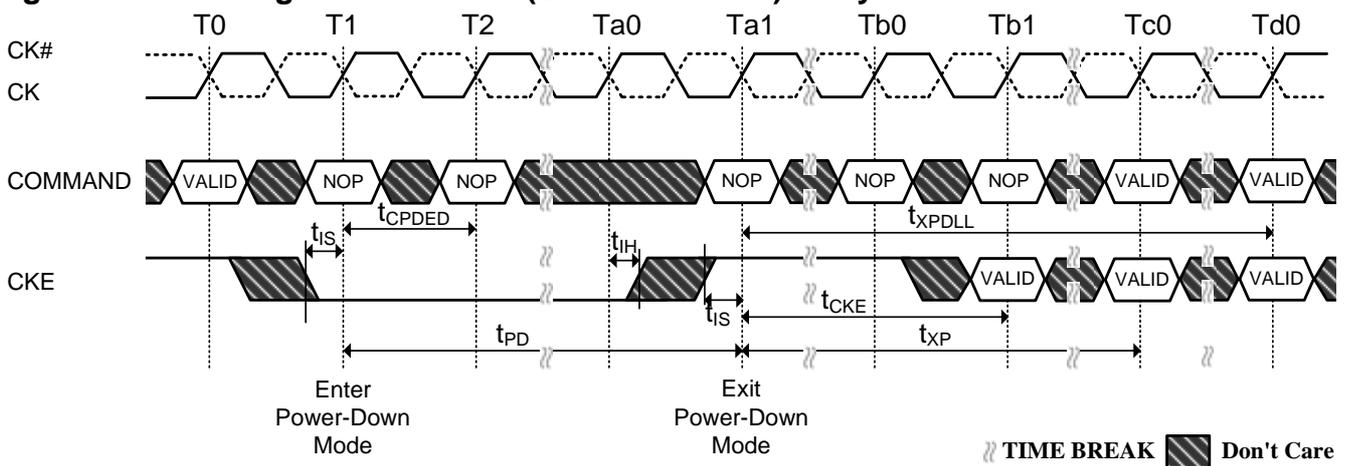
**Figure 61. Refresh Command to Power-Down Entry**
