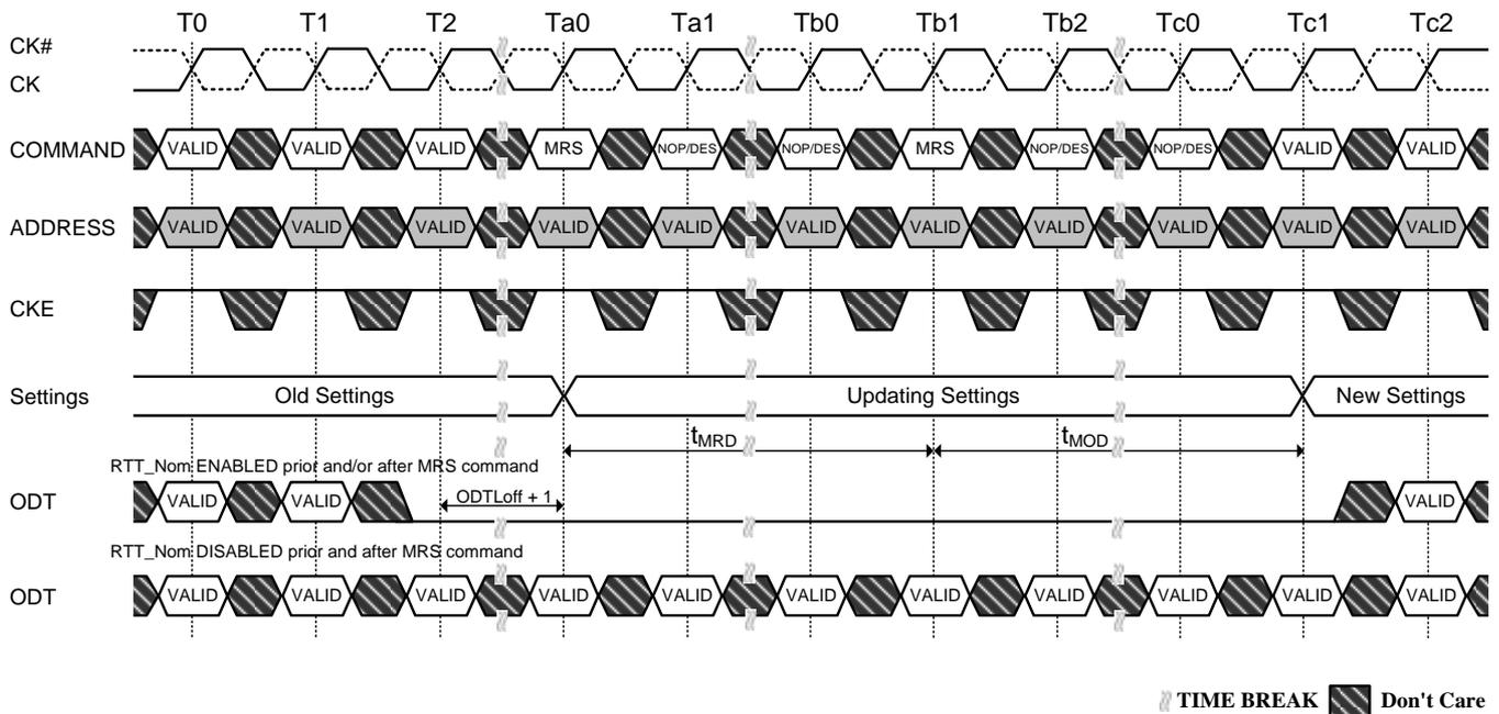
The MRS command to Non-MRS command delay,  $t_{MOD}$ , is require for the DRAM to update the features except DLL reset, and is the minimum time required from an MRS command to a non-MRS command excluding NOP and DES shown in Figure of  $t_{MOD}$  timing.
