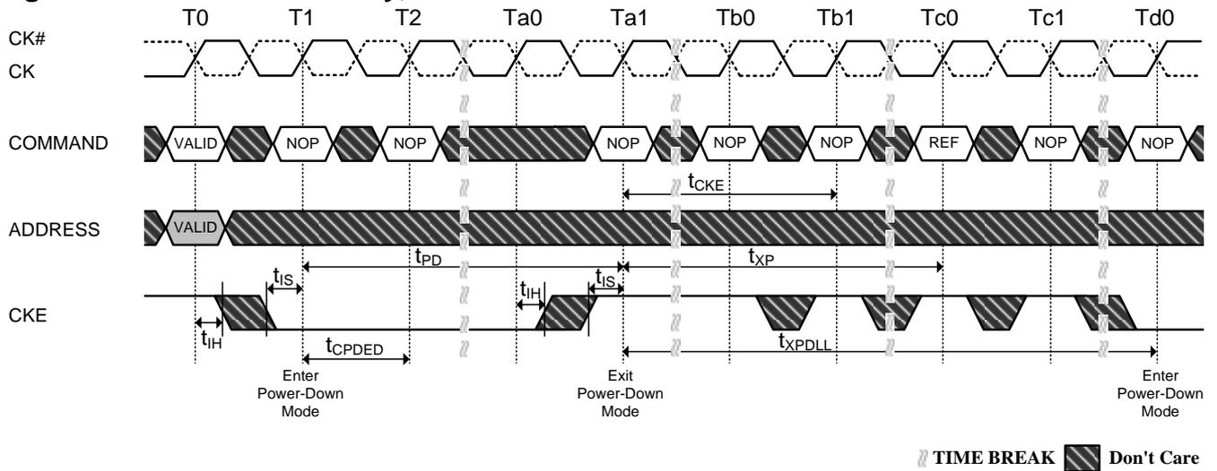
**Figure 79. Power-Down Entry,Exit Clarifications-Case 3**
