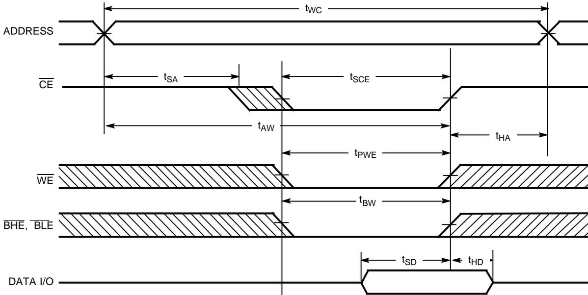
Figure 6. Write Cycle No. 2 ( $\overline{\text{BLE}}$  or  $\overline{\text{BHE}}$  Controlled)
