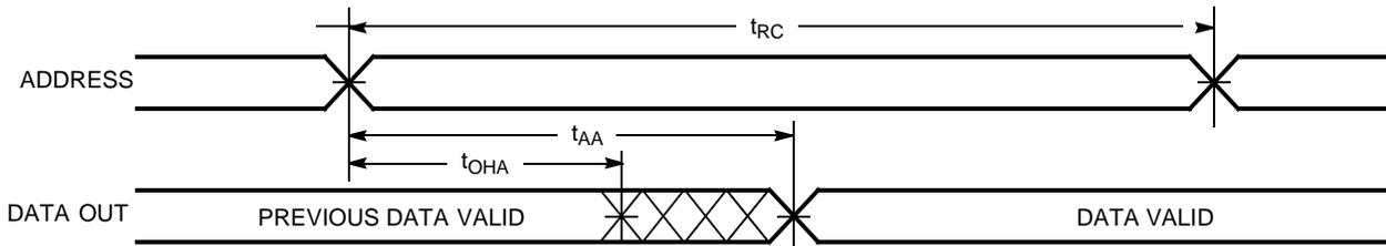
Figure 4. Read Cycle No. 2 ( $\overline{OE}$  Controlled) [11, 12]
