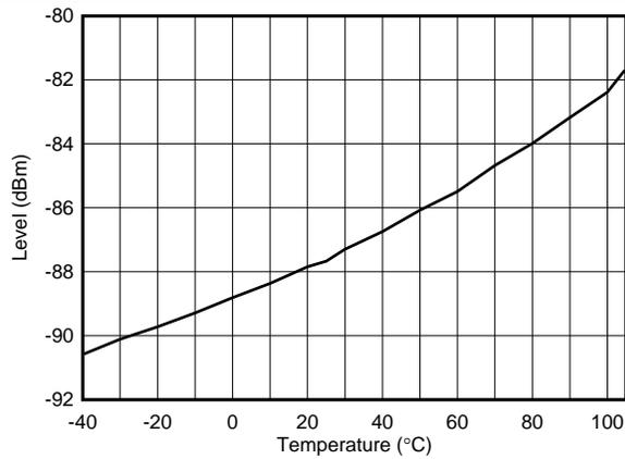
Figure 4-9. RX Sensitivity vs Temperature
