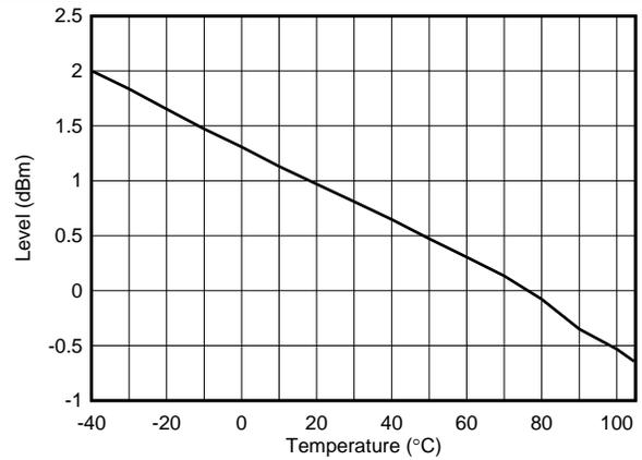
Figure 4-10. TX Power vs Temperature
