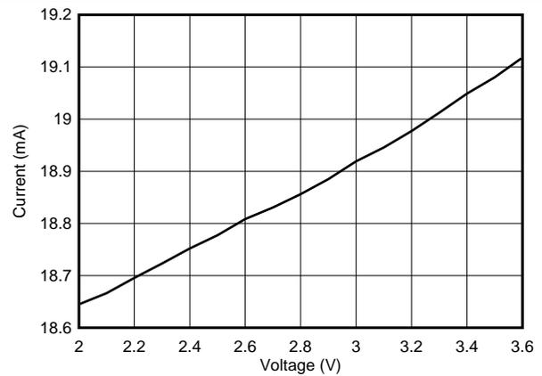
Figure 4-12. TX Current vs Supply Voltage
