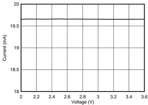
Figure 4-11. RX Current vs Supply Voltage
