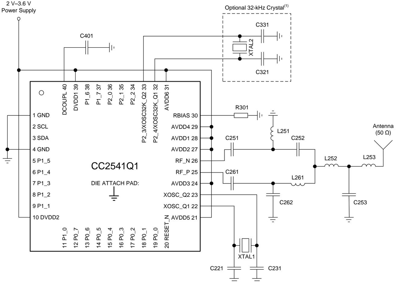
(1) 32-kHz crystal is mandatory when running the BLE protocol stack in low-power modes, except if the link layer is in the standby state (Vol. 6 Part B Section 1.1 in [1]).
