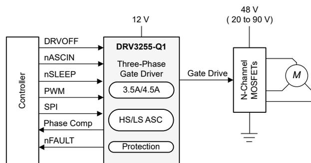
Figure 3-1. Simplified Schematic
