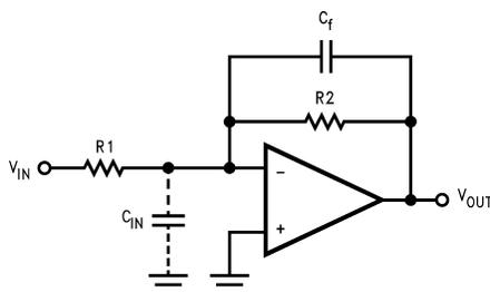
Figure 24. Canceling the Effect of Input Capacitance
