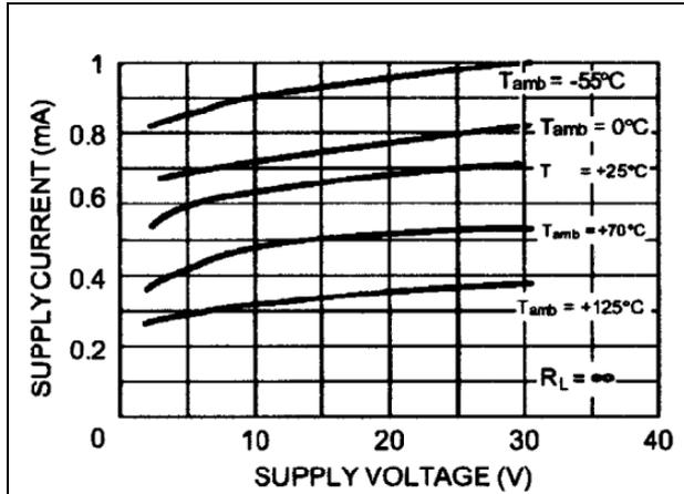
Figure 3. Input current versus supply voltage
