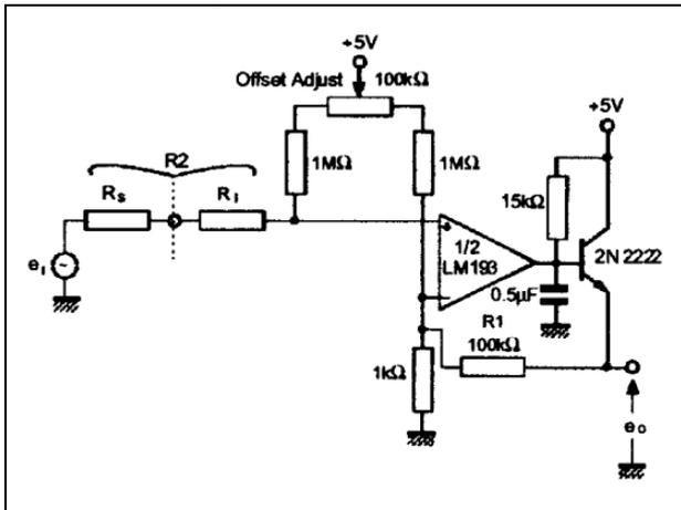
Figure 14. Zero crossing detector (single power supply)
