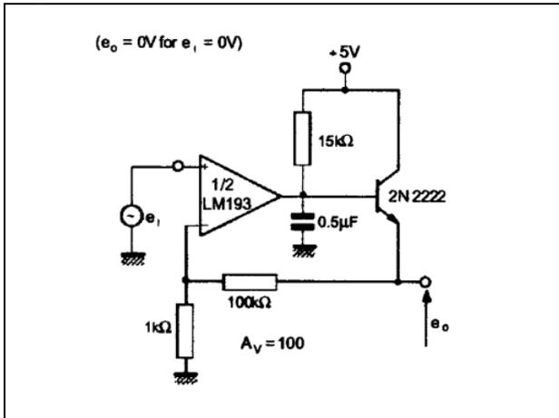
Figure 12. Transducer amplifier
