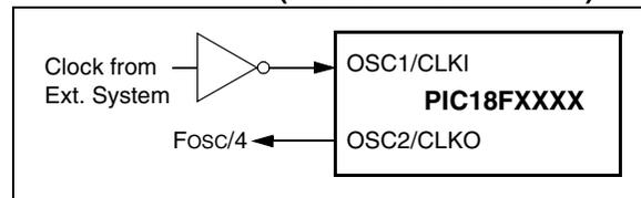
The ECIO Oscillator mode functions like the EC mode, except that the OSC2 pin becomes an additional general purpose I/O pin. The I/O pin becomes bit 6 of PORTA (RA6). Figure 2-4 shows the pin connections for the ECIO Oscillator mode. When operated in this mode, parameters D033A and D043A apply.
