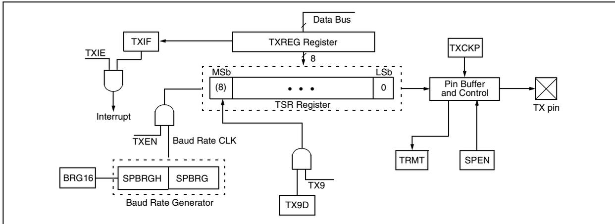
**FIGURE 18-4: ASYNCHRONOUS TRANSMISSION, TXCKP = 0 (TX NOT INVERTED)**
