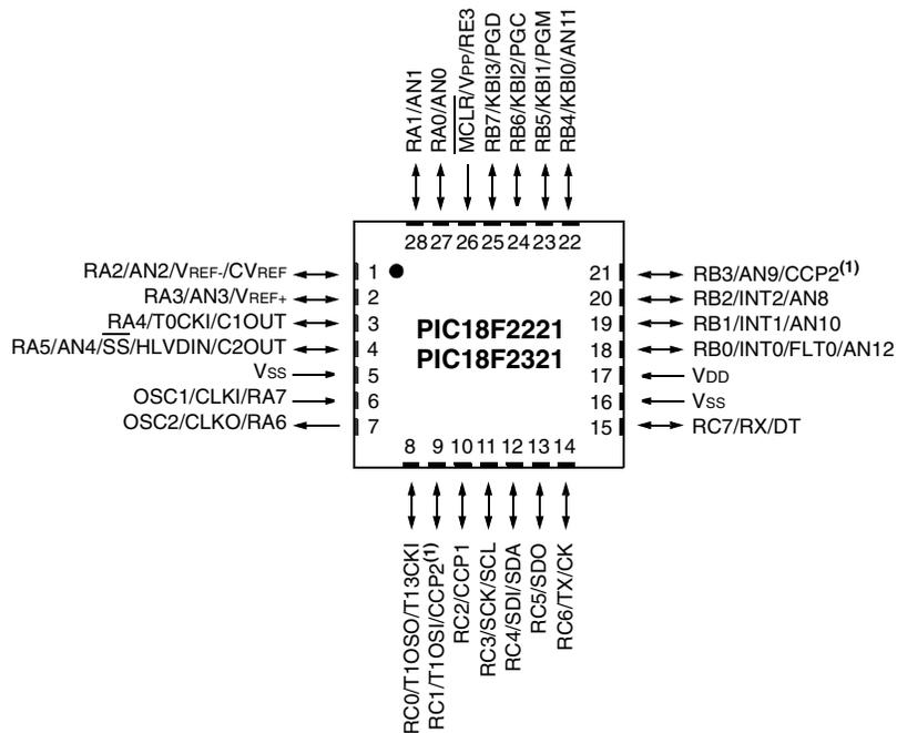
**Note 1:** RB3 is the alternate pin for CCP2 multiplexing.
