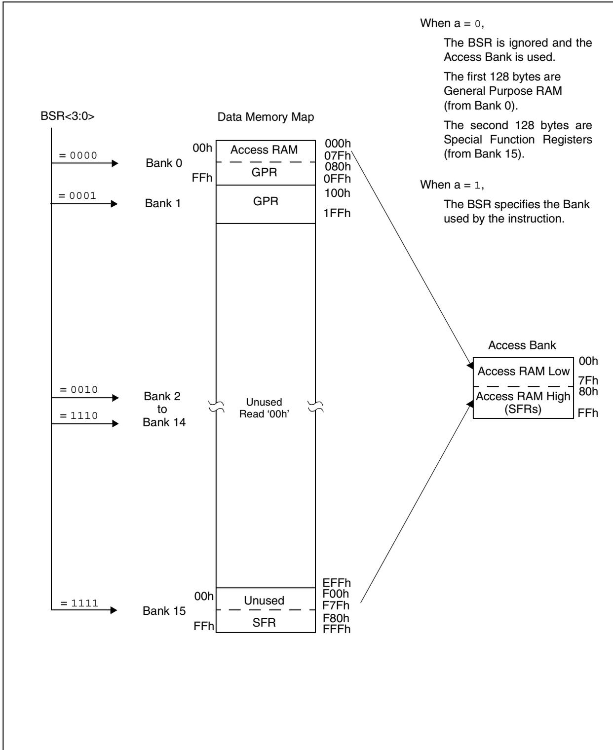
**FIGURE 5-6: USE OF THE BANK SELECT REGISTER (DIRECT ADDRESSING)**
