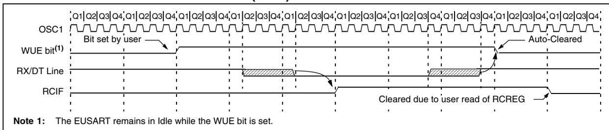
**FIGURE 18-9: AUTO-WAKE-UP BIT (WUE) TIMINGS DURING SLEEP**
