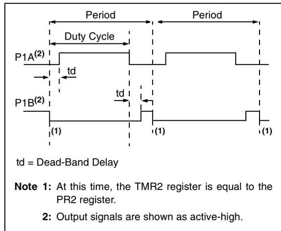
**FIGURE 16-5: EXAMPLES OF HALF-BRIDGE OUTPUT MODE APPLICATIONS**
