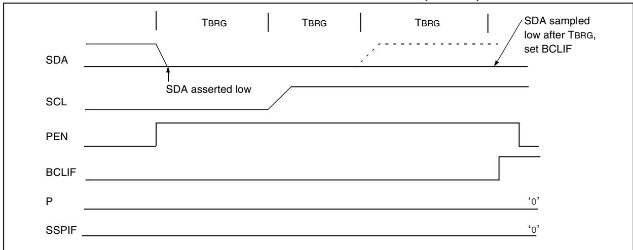
**FIGURE 17-34: BUS COLLISION DURING A STOP CONDITION (CASE 2)**
