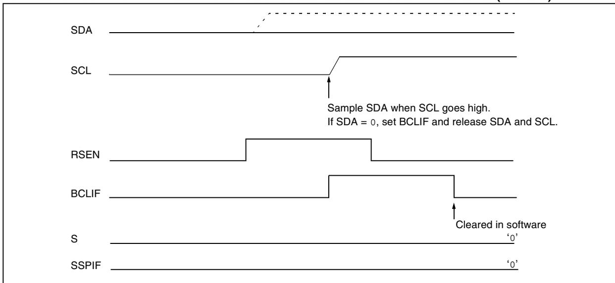
**FIGURE 17-32: BUS COLLISION DURING REPEATED START CONDITION (CASE 2)**
