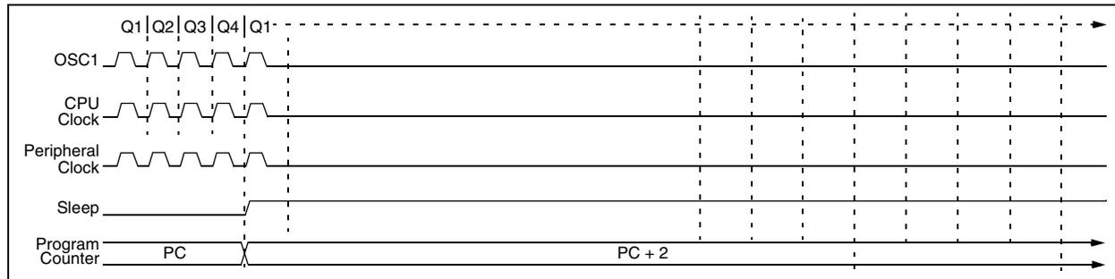
**FIGURE 3-6: TRANSITION TIMING FOR WAKE FROM SLEEP (HSPLL)**
