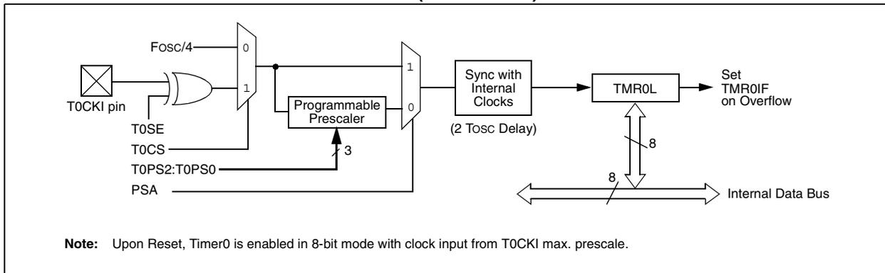
**FIGURE 11-2: TIMER0 BLOCK DIAGRAM (16-BIT MODE)**
