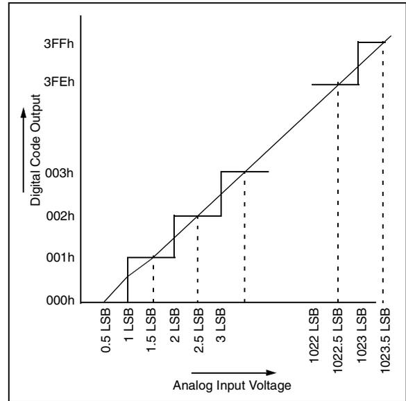
**FIGURE 19-3: ANALOG INPUT MODEL**
