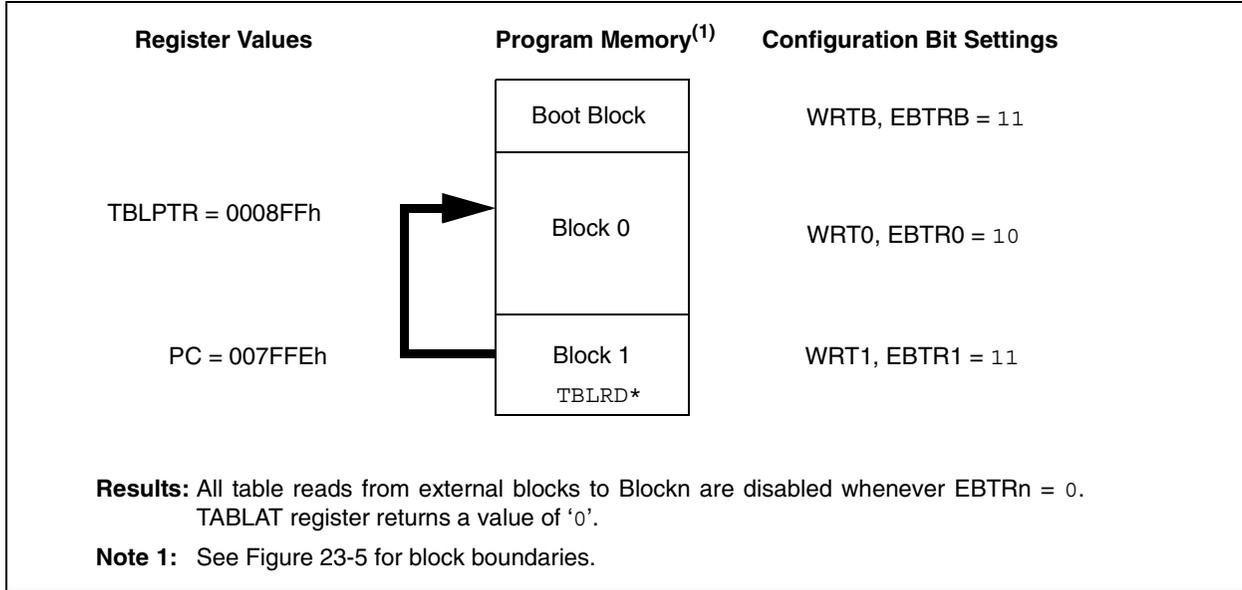
**FIGURE 23-8: EXTERNAL BLOCK TABLE READ (EBTRn) ALLOWED**
