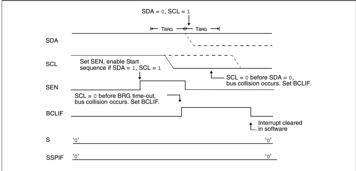
**FIGURE 17-30: BRG RESET DUE TO SDA ARBITRATION DURING START CONDITION**
