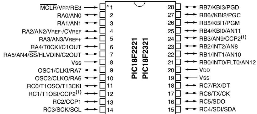
**Note 1:** RB3 is the alternate pin for CCP2 multiplexing.
